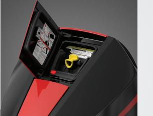
Industry-exclusive Top Cowl Service Door simplifies routine maintenance with easy oil checks and oil fills without removing the cowl. Graphic, hour-based maintenance decals under the cowl for easy access to all regular powerhead maintenance points. Maintenance-free valve-train for life of the engine.
